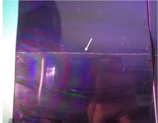
Figure 1. The typical failure phenomenon that occurs when the foldable screen is rapidly opened in -20^{\circ}\text{C} environment after being bent for several hours.
